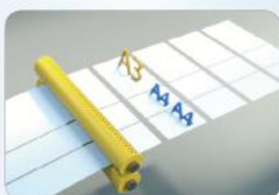
双回旋同步剪切 Twin Rotary Knife Synchronize Sheeting
